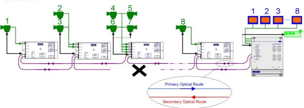
If multiple breaks occur, operation is maintained with all the units still physically connected to the receiver. For the scenario shown below camera signals and control would now be lost from cameras 1, 2 and 3 as there is now no physical connection between the transceivers and the receiver. However operation of cameras 4,5,6,7 and 8 remains fully functional.
