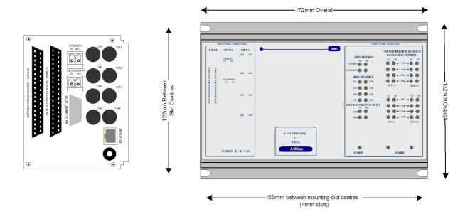
The **AMG3707-DR** is a standalone data insert unit designed to transmit and receive up to 16 data or audio signals over two singlemode fibres with Dual Redundant operation. The 16 data/audio channel interfaces, whether RS-232, RS-422, RS-485, 20mA, TTL, Contact Closure, Lonworks or Audio, are defined at manufacture by the addition of daughter boards fitted onto the Data Expansion Board B.
